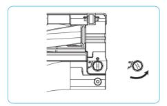
**Step 1** Detach the Floor Tool from the vacuum. Use the notch to turn the latch's lock counter-clockwise.
