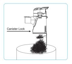
Step 1 Detach the Canister from the Main Body as seen in Section 5.2. Hold the Canister over a wastebin and press the Canister Lock to open it. Empty the bottom.
