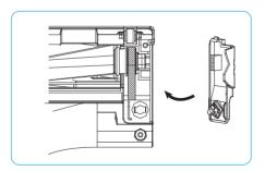
Step 5 Replace the agitator, pull the belt back on the right side, and replace the latch.
