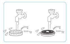
Step 3 Rinse one or both parts of the filter if desired. After rinsing, allow 24 hours' time for the filter to dry.
