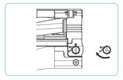
**Step 6** Use the notch to turn the latch's lockclockwise.
