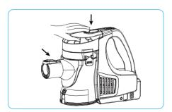
**Step 1** Press the Body Lock to remove the Canister from the Main Body of the vacuum.
