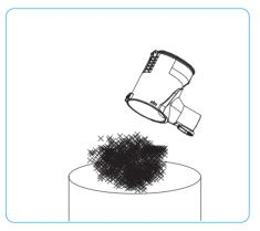
**Step 3** Hold the Canister over a waste bin and empty the top.
