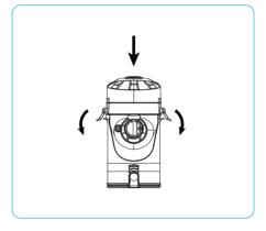
Step 4 Return the top and connected Filtration System to the Canister. Fold the Canister clips down to refasten the top. Reattach the Canister to the Main Body as seen in Section 5.2.
