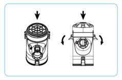
**Step 4** Reinstall the filter and top of the Canister then reattach the Canister to the Main Body as seen in Section 5.2.
