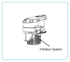
**Step 2** Lift the Canister clips to unfasten the top and connected Filtration System. Set these parts aside.
