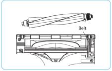
**Step 4** Lift the agitator out, hold it over a waste bin, and shake off any dust. Pull or cut out any entangled debris as needed.
