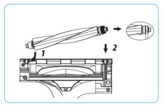
**Step 3** Lift the agitator up slightly and carefully pull the belt off.
