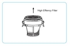
**Step 2** Take out the Filter and separate the mesh from the sponge.
