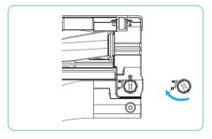
**Step 6** Use the notch to turn the latch's lock clockwise.
