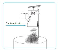
Step 1 Detach the Canister from the Main Body as seen in Section 5.2. Hold the Canister over a waste bin and press the Canister Lock to open it. Empty the bottom.
