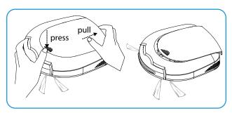
**Step 1.** Using the arrows as a guide, gently press on the top cover and pull it to remove it.
