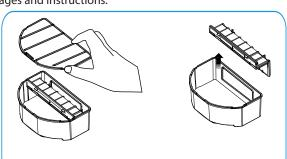
**Step 1.** Remove the dustbin and its lid to locate the filter, then remove the filter.
