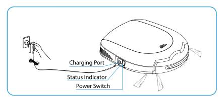
**Step 1.** Locate the charging port on the side of the RolliCute near the power switch.
