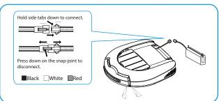
**Step 2.** Locate the battery cords and the RolliCute's cords. Hold down the tabs on each and connect the two.
