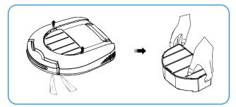
Step 2. Locate the dustbin. Using the notches at either side, grasp the dustbin and carefully lift it out of the RolliCute.
