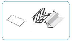
**Step 4.** Using a new or cleaned and dried filter, push it onto the filter bracket's pegs.
