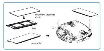
Step 4. Optionally, attach a microfiber cleaning cloth to its base. Then, attach the base to the underside of the RolliCute. The cloth may be lightly dampened before attachment if desired.
