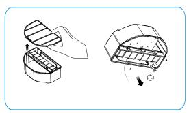
**Step 1.** After removing the dustbin, push the edges of the lid up to lift it off and remove it.
