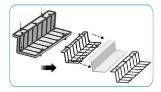
**Step 2.** Push open each of the four tabs to separate the filter brackets.
