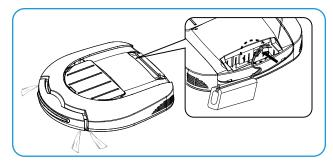
**Step 3.** Carefully push the connected cords into the corner slot.
