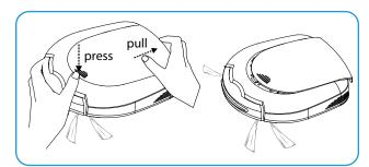
**Step 1.** Using the arrows as a guide, gently press on the top cover and pull it to remove it.
